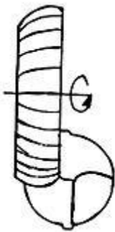
Fig. Cutting of drill flutes
